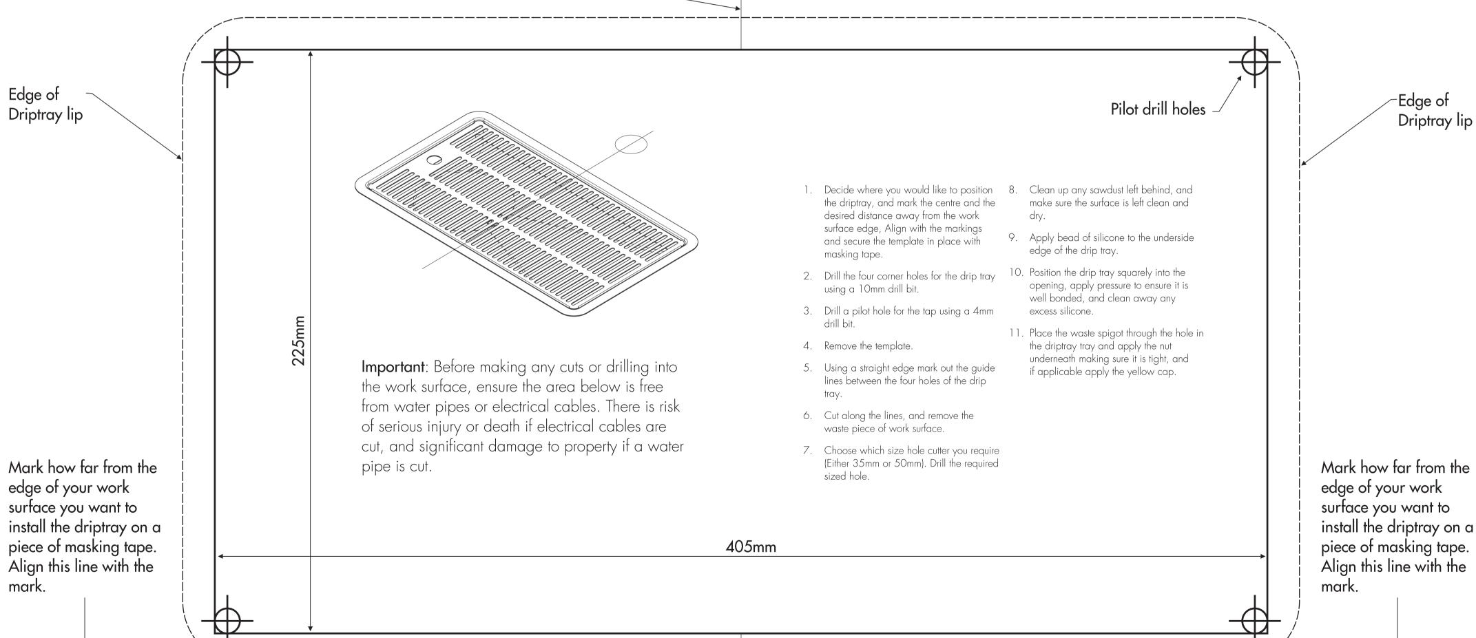
Ensure this line is parallel to front edge of the work surface.
