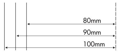
Choose how far from the edge of your work surface you want to install the Driptray, and mark this on a piece of masking tape.
