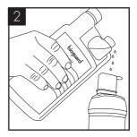
Add 25 ml of Bioguard Internal Sanitisation fluid to a clean and empty service filter cartridge and connect to the machine.
