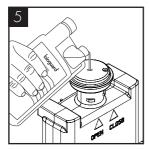
Remember to include the drip tray. Empty the Waste Overflow system and flush through with a small amount of sanitisation fluid if needed
