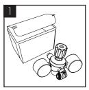
Unpack CO<sub>2</sub> Regulator and fit elbow fitting to spigot outlet.
