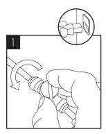
Connect and turn on the water supply. Then connect the power supply.
