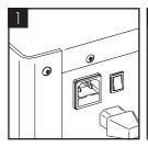
Connect the unit to the electricity supply and ensure unit is switched on.
