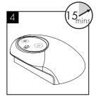
Allow the machine to stand for 15 minutes for the initial chilling and heating process to complete.
